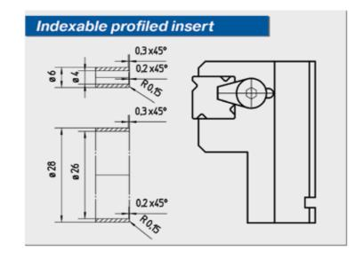
This tried and tested insert from the tube chamfering head with its four equal cutting edges can also be used on an adjustable holder and a tool head from stock. This makes it possible to economically machine related items with the same contour and various pipe diameters.
