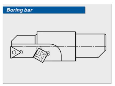
A **boring bar** can also be clamped in the center bore of the end finishing tool instead of a clamping sleeve for drills, for additional boring routines.
