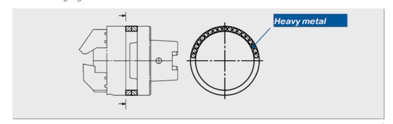
→ Tube chamfering head / Paring tool
