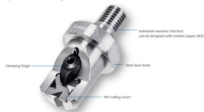
The two-part mold consists of a basic holder, which can be manufactured with individual shank designs on request, and a replaceable mold plate with up to four cutting edges. The unused cutting edges lie safely protected in a comprehensive plate seat. The real innovation lies in the special design of the cutting geometry of the forming plates. Whether classic facing and chamfering or a specific profile contour, many things can be produced in a single operation.
