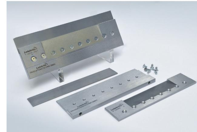
Carbide inserts with a basic thickness of 2 mm are ground in A-dimension (carbide thickness) in accordance with the workpieces that will be ground. In this example, it is 0.5 mm. Various inserts can be stocked and changed by the customer.
